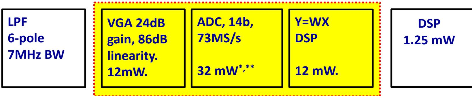
\*Analog Devices AD9269 = 44mW Power Dissipation at 20 MSPS/Channel (36 fJ/conversion)
