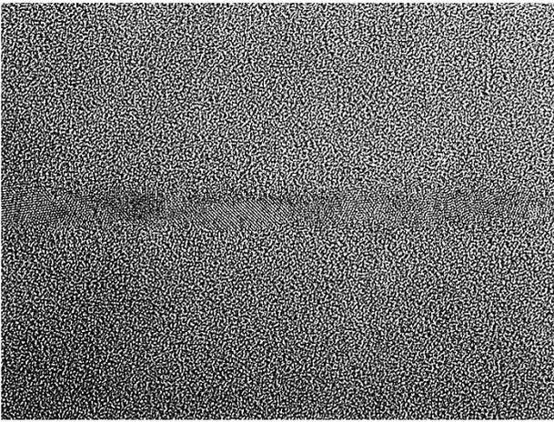
Fig. 6. Cross-sectional TEM photograph of the channel poly-Si.
