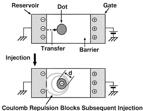
Fig. 1. The schematic view of the single-electron box.
