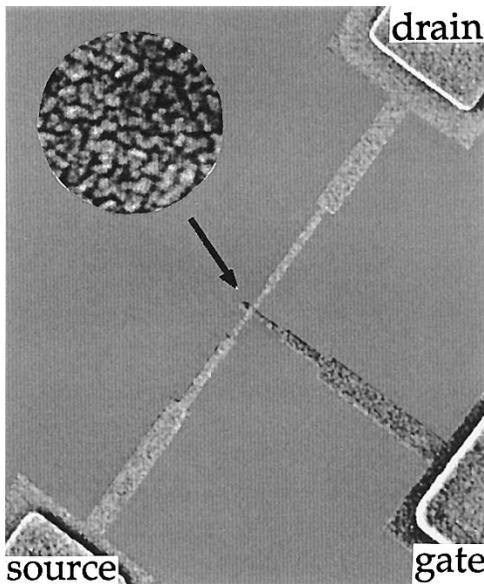
Fig. 7. The SEM microphotograph of the fabricated memory. Nano-Si is sandwiched by amorphous silicon dioxide.
