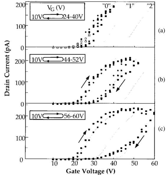
Fig. 9. Measured drain current versus gate voltage. The drain-source voltage is 50 mV. The gate-voltage sweep rate is 4 V/min. The maximum gate voltage in a sweep loop is: (a) 24 V( $\circ$ ), 28 V( $\square$ ), 32 V( $\blacklozenge$ ), 36 V( $\bullet$ ), 40 V( $\blacksquare$ ); (b) 44 V( $\blacklozenge$ ), 48 V( $\bullet$ ), 52 V( $\blacksquare$ ); and (c) 56 V( $\bullet$ ), and 60 V( $\blacksquare$ ).
