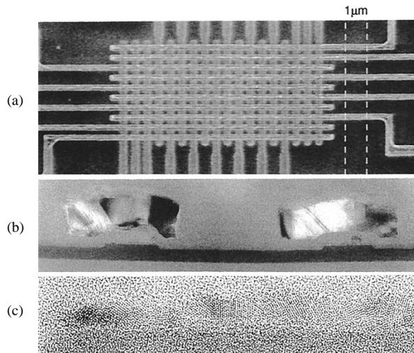
**Fig. 12.** Microphotograph of an  $8 \times 8$ -bit memory-call array: (a) SEM view showing horizontal word lines and vertical data/source lines; (b) cross-sectional TEM view across word line and channel; and (c) enlarged TEM view of nano-Si. Word-line pitch is  $0.55 \mu\text{m}$ .
