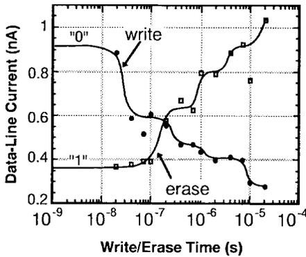
Fig. 15. Write/erase characteristics. The word/data line voltage for current measurement is 1 V/1 V, respectively.
