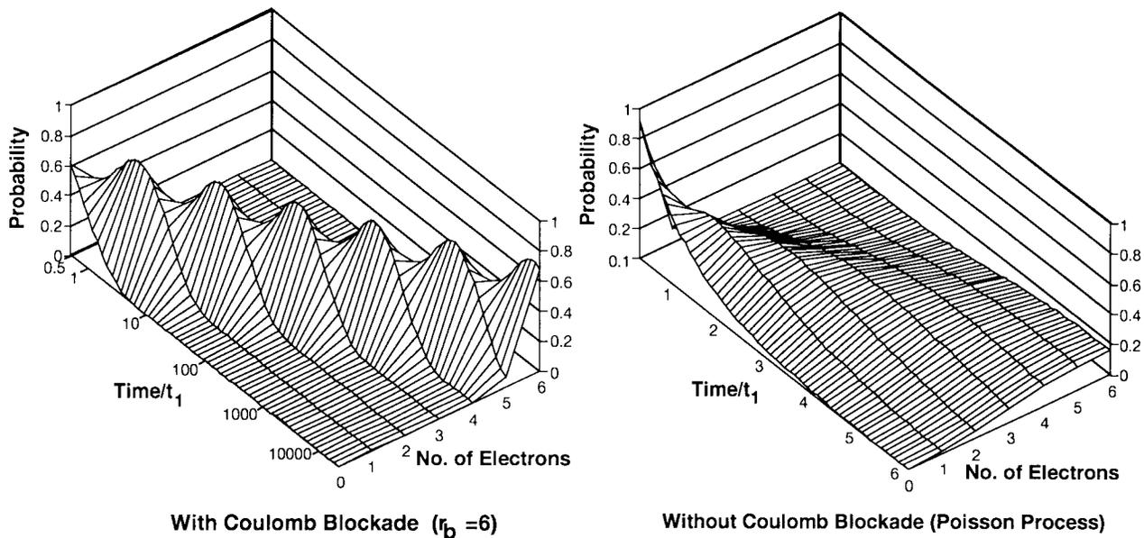
Fig. 22. Simulated time evolution of probability distribution function, which demonstrates the self-stabilizing nature of the distribution under the Coulomb blockade condition.
