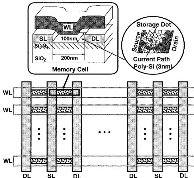
Fig. 10. Schematic structure of ladder-shaped Coulomb memory cell array. Word line (WL), data line (DL), and source line (SL) are poly-Si.
