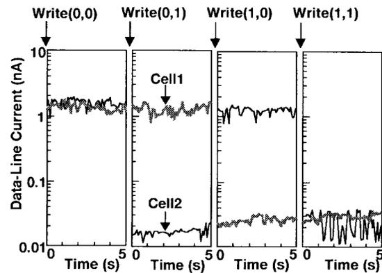
**Fig. 13.** Repeated erase/write/read of two memory cells sharing word line and source line. Word/data-line voltages are those in Fig. 11, except read is at  $0.1 \text{ V}/1 \text{ V}$ , respectively. The write/erase is completed within 1 ms.
