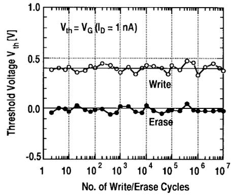
Fig. 16. Endurance characteristics versus write/erase cycles.
