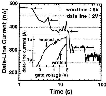
Fig. 14. Data-line current during write at 9 V showing one-by-one trapping events. The trapping time constant gets exponentially longer each time an electron is trapped, which directly shows Coulomb blockade illustrated in Fig. 1.
