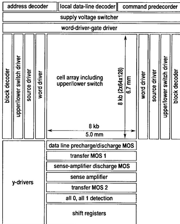
Fig. 26. Block diagram of the fabricated 128-Mbit memory prototype.
