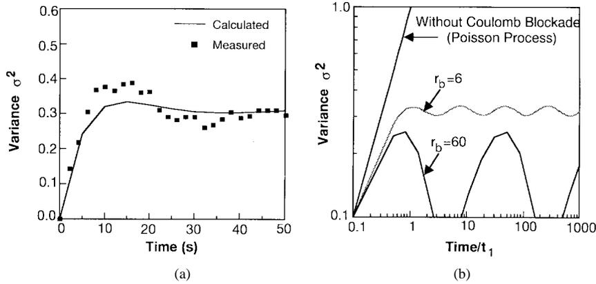
**Fig. 21.** Comparison of electron-count variance between experiment and calculation: (a) shows good agreement between the measured result and the simulation result; it also shows sub-one-electron control of electron count in this device and (b) shows grand behavior of the simulation result and the dependence on Coulomb blockade factor  $r_b$ .
