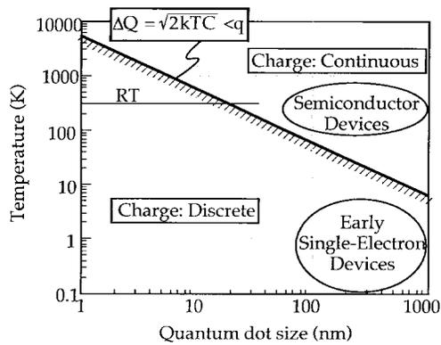
Fig. 2. Conditions for the Coulomb blockade. The self-capacitance of uniformly charged sphere is assumed in the calculation.
