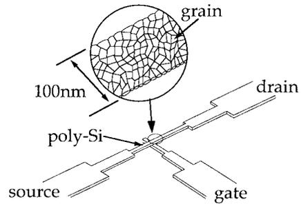
Fig. 8. Fabricated nano-Si memory structure and enlarged active region.
