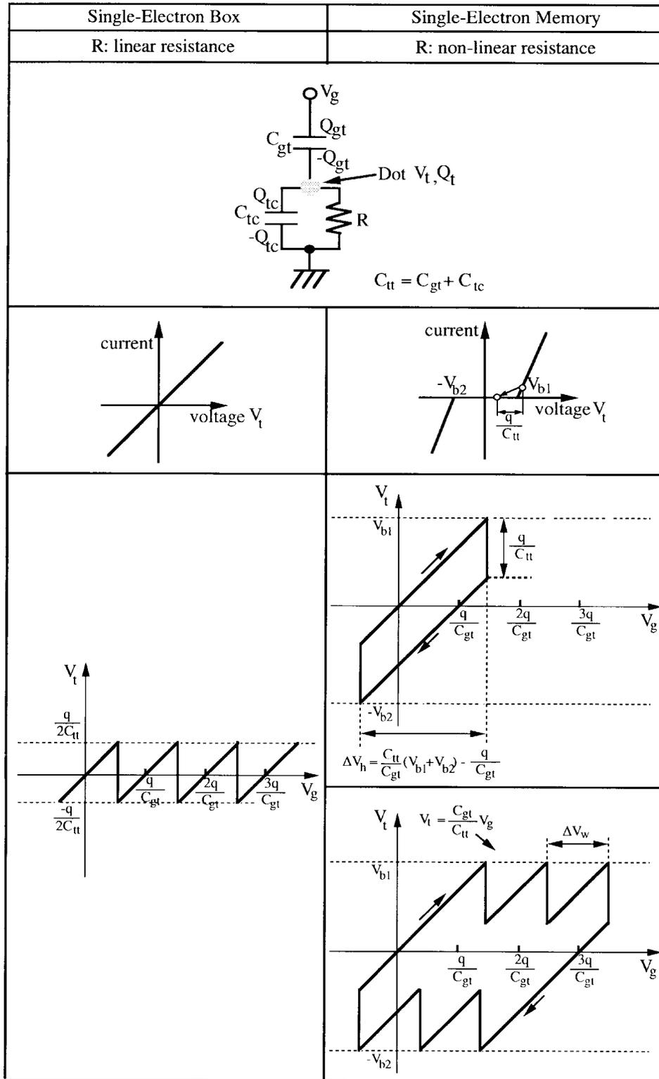
**Fig. 3.** Comparison between the single-electron box and single-electron memory. Nonlinear resistance characterized by the threshold voltages  $V_{b1}$  and  $V_{b2}$  is essential for the memory operation: (a) circuit; (b) IV curve of resistance  $R$ ; (c) storage node potential.
