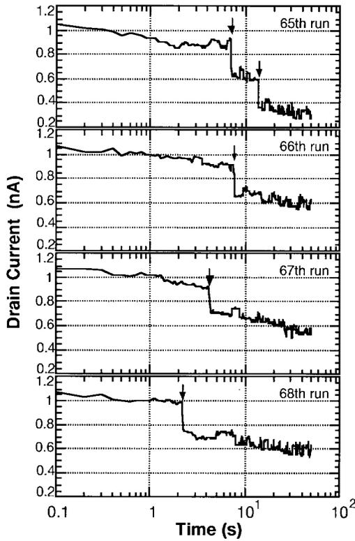
Fig. 18. Real-time electron counting measurement at write voltage of 12 V. The electron injection into a storage dot is indicated by an arrow. Four successive runs are depicted from 100 runs. An abrupt current reduction corresponds to 0.6-V threshold shift. The drain voltage was 10 mV.
