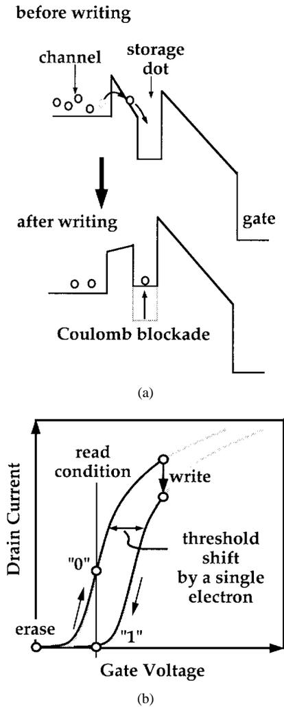
Fig. 4. (a) Schematic energy diagram for the proposed single-electron memory. (b) The schematic current-voltage curve of the memory device.
