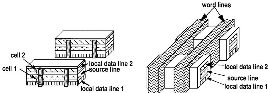
Fig. 23. Vertically united cell structure, which integrates two cells in a contact area. The nano-Si is deposited on the sidewall of the data line and source line stack.
