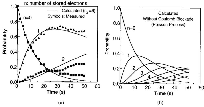
**Fig. 20.** The time dependence of probability distribution of stored electrons: (a) shows the experimental results combined by the Coulomb blockade model calculation result and (b) shows different behavior when we neglect Coulomb blockade (this corresponds to Poisson process.)
