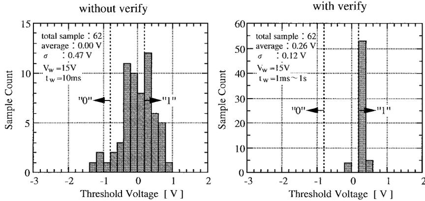
Fig. 17. Threshold voltage distribution after write in an array.
