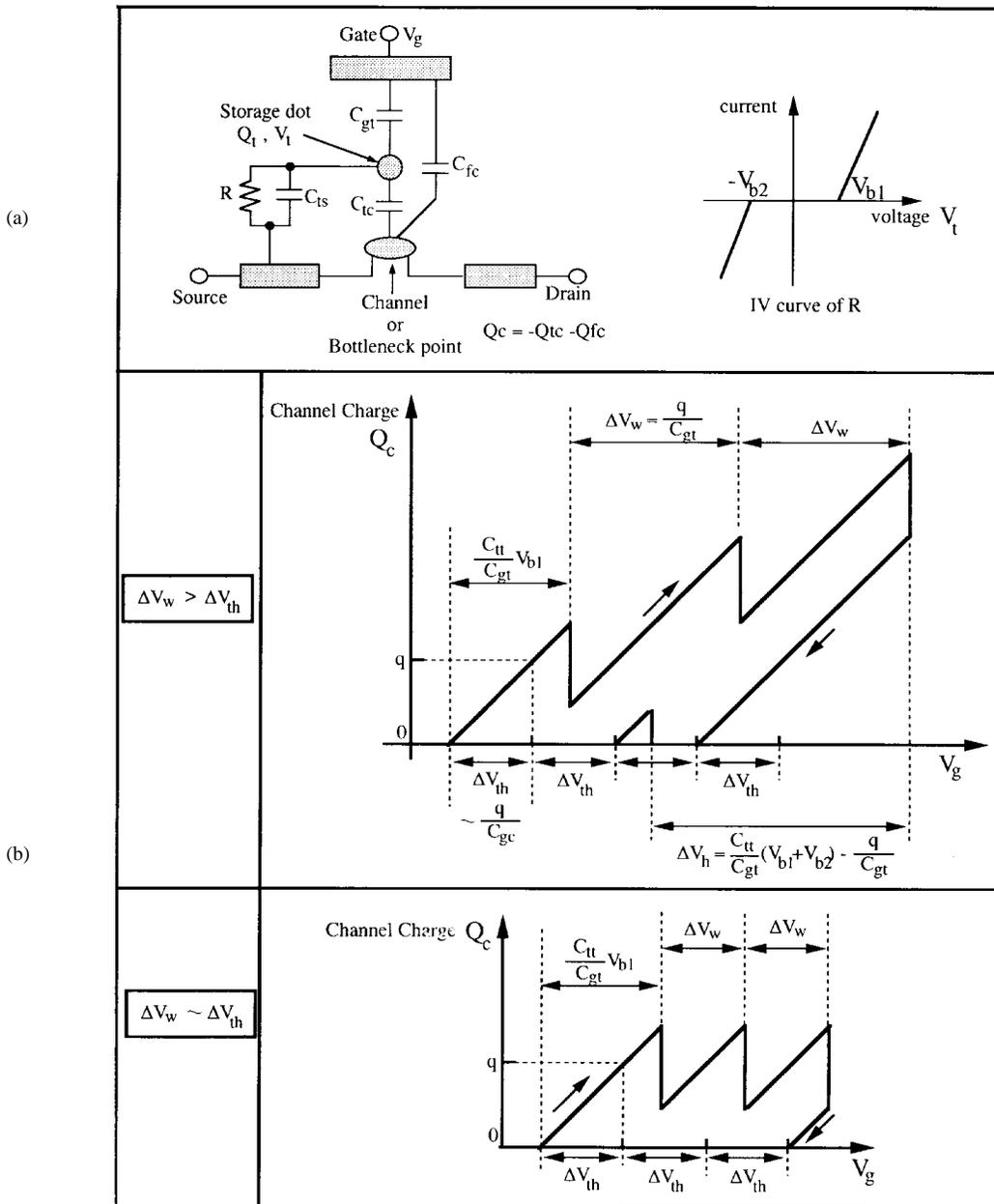
**Fig. 5.** The equivalent circuit and typical behavior of the proposed single-electron memory. Two types of behaviors are possible depending on the single-electron write period  $\Delta V_w$  and threshold voltage shift  $\Delta V_{th}$ .  $\Delta V_h$  is the width of the hysteresis: (a) equivalent circuit and (b) channel charge versus gate voltage.
