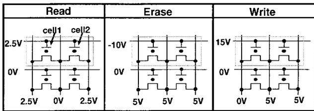
**Fig. 11.** Memory-cell array operating voltages. Four cells are shown as an example. Target cells are cell1 and cell2, and the other two cells are not target cells but are inevitably biased in this array organization.
