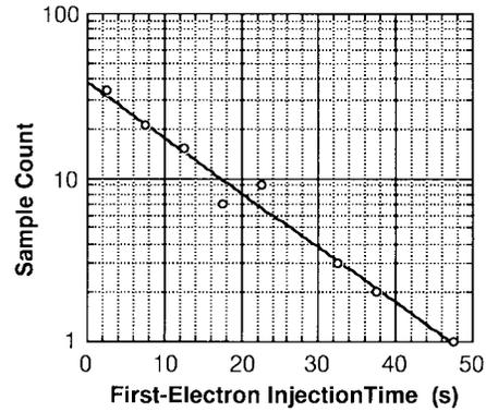
Fig. 19. The histogram of the first-electron injection time. The results fit well with the exponential decay expected for single-time constant process. The time constant is 12.9 s.
