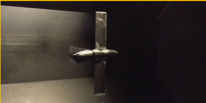
A bird-like model made of carbon fiber sits in the DWT test section, ready to be measured (Davis & Spedding, 2016).
