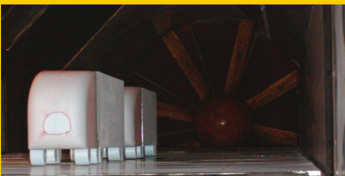
Two model trucks on a platform that removes the boundary layer to mimic movement over a stationary road (Browand, 2008).
