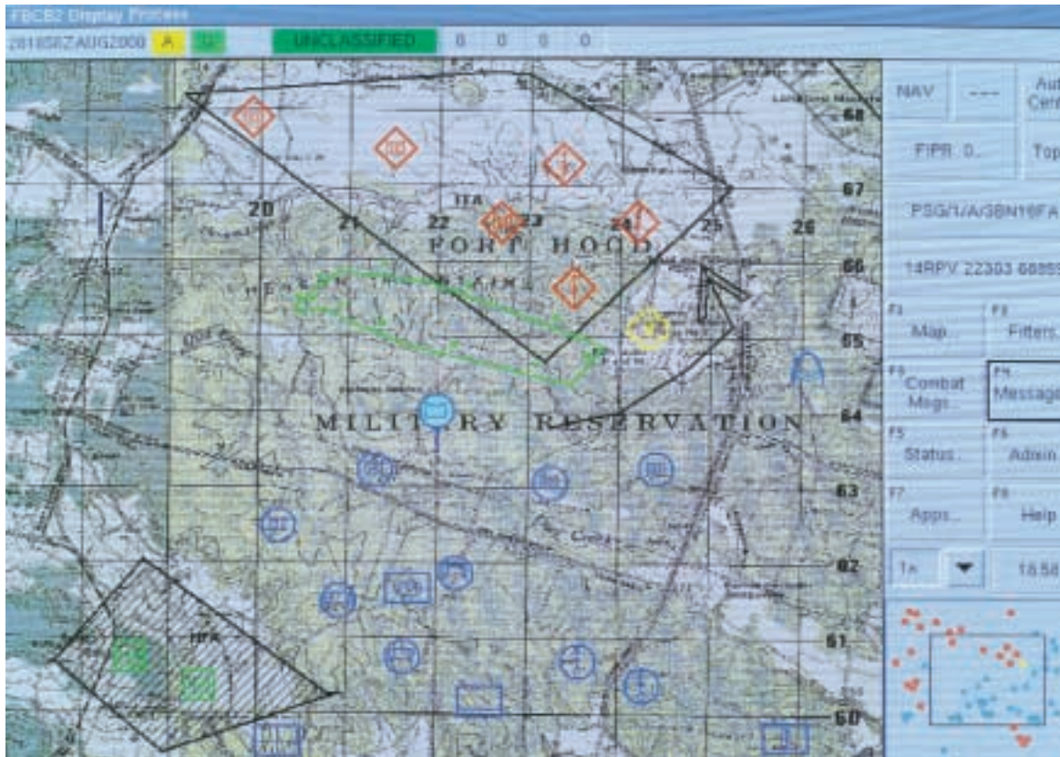
The FBCB2 touchscreen displays in color the location of friendly and enemy forces, providing soldiers and commanders with near-real-time battlefield information.
