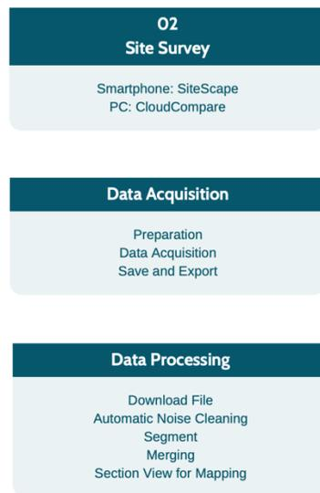
Figure 4-30: Heritage conservation survey by smartphone workflow diagram
