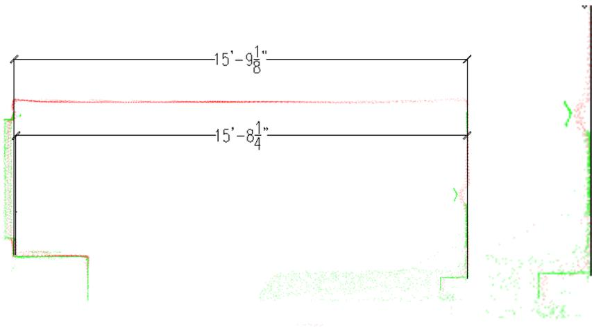
Figures 5-29 and 5-30: Low density iPhone scan (red) and RTC 360 scan (green) section 1 (left), and detail (right).
