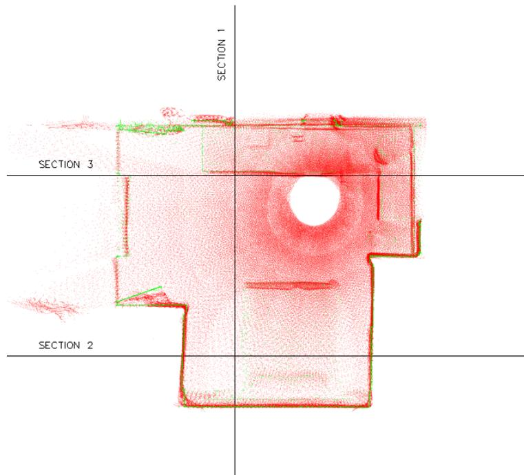
Figure 5-13: Section layout on point clouds
