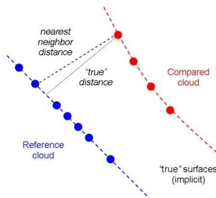
Figure 4-86: CloudCompare distance computation working principle
