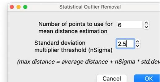
Figure 4-39: SOR (Statistical Outlier Removal) setup
