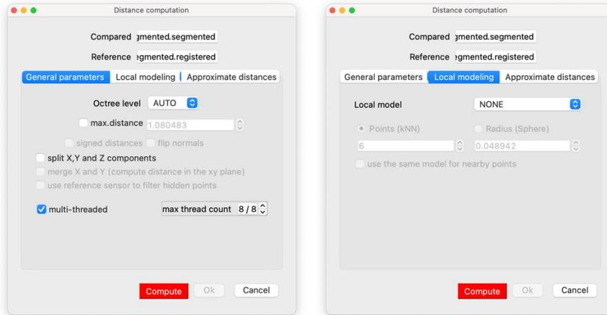
Figure 4-81: Distance computation parameter setup
