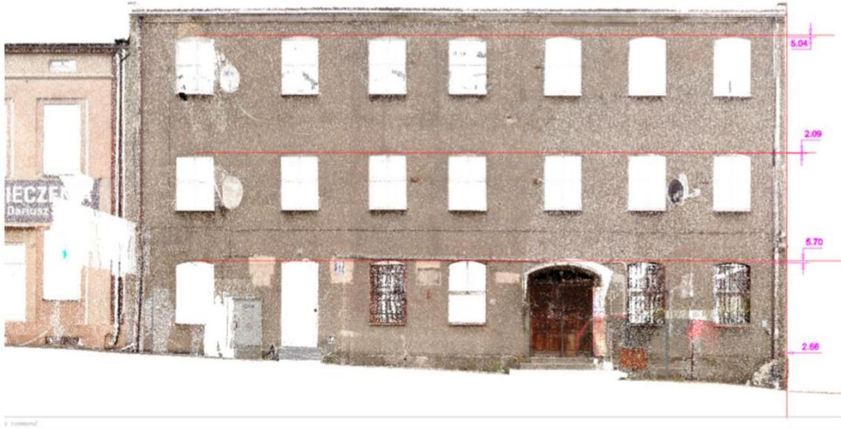
Figure 2-11: TSL scanned data in Autocad measuring deformation of front wall (Nowak et al., 2020).
