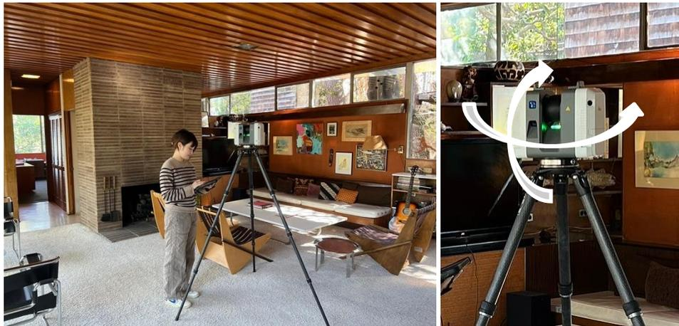
Figures 5-3 and 5-4: Professional scanner scan and moving path
