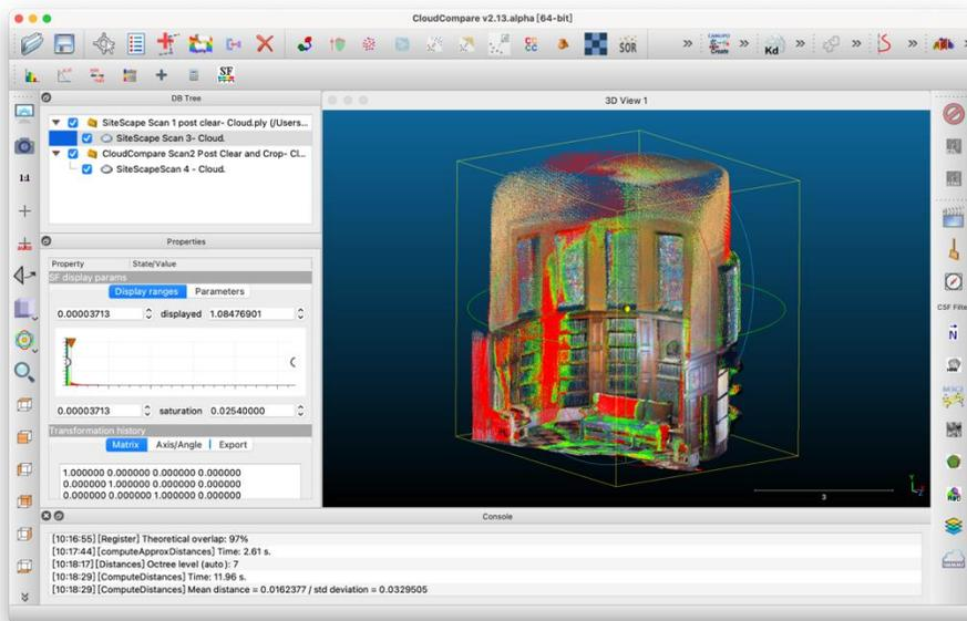
Figure 4-85: Scan 3 and Scan 4 distance with saturation 1 inch. Distance reduced from red to green to blue.
