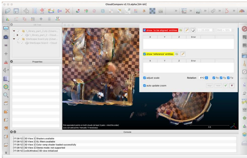
Figures 4-64, 4-65, and 4-66: Align two clouds by picking four points tool, select to-be-aligned entities window, and alignment interface
