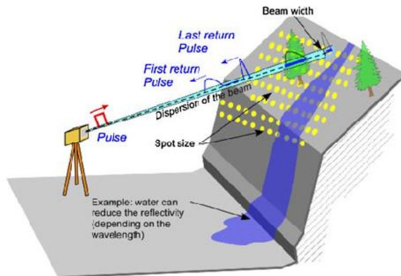
Figure 1-14: Principles of laser scanner data acquisition, showing the example of TLS (Jaboyedoff et al., 2012)
