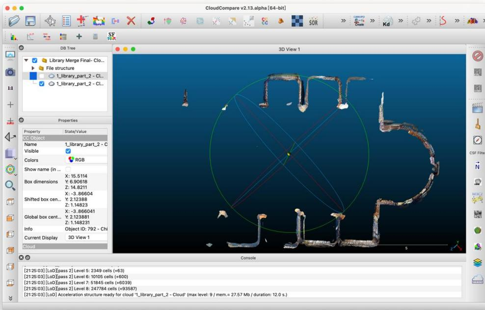
Figures 4-71 and 4-72: Creating a slice of structure with segment tool, bird eye view of the floor plan
