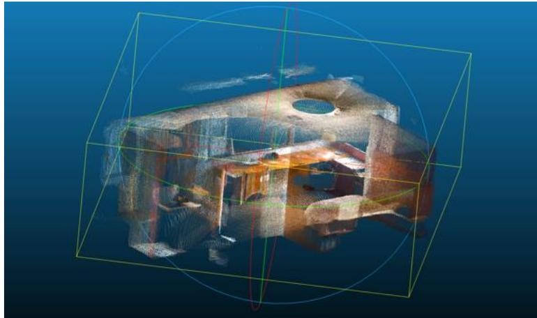
Figure 5-11: Three smartphone scans (leveled, upper and lower angled) merged with CloudCompare
