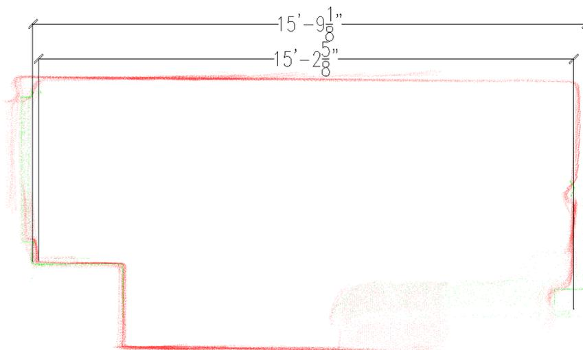
Figure 5-31: Merge of high point density scans from smartphone aligned with professional scanner point clouds
