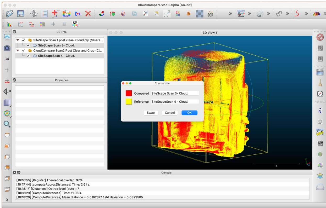
Figure 4-80, *Scan 4* as Reference and *scan 3* as Compared in CloudCompare cloud to cloud distance function
