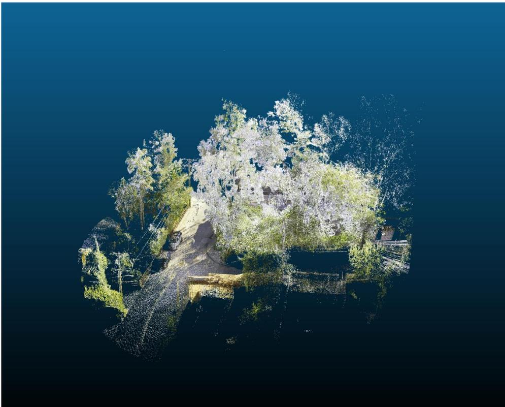
Figure 6-12: RTC 360 scanned outdoor environment at Reunion House
