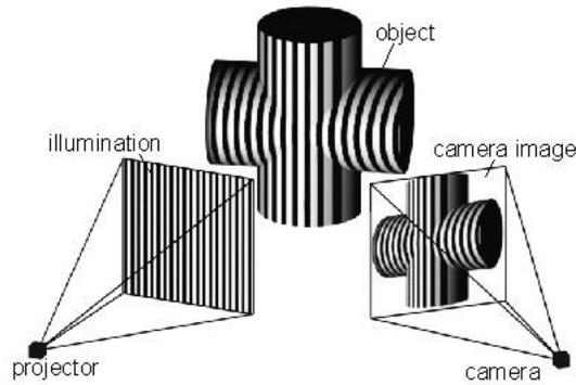
Figure 1-12: Working principle of Structured Light scanners (Bitfab, 2022)
