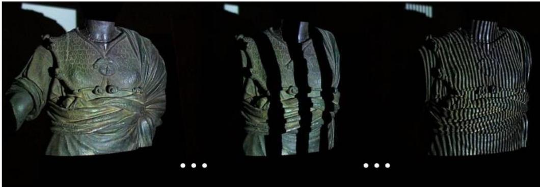
Figure 2-10: Structured light scanning on the Minerva case study (Rocchini et al., 2001).
