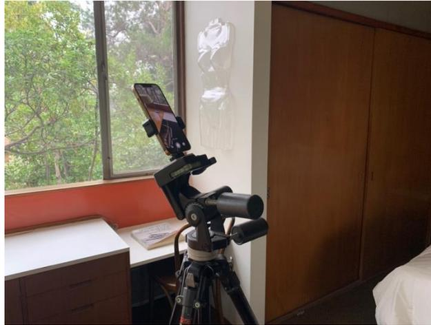
Figure 4-18: The smartphone device on tripod with an angle facing down
