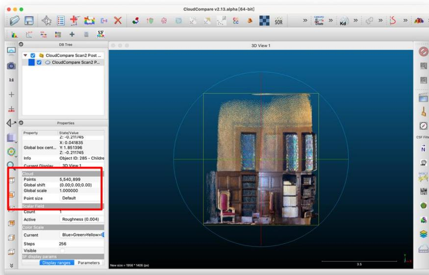
Figure B-12: Number of points for *scan 2 filter*
