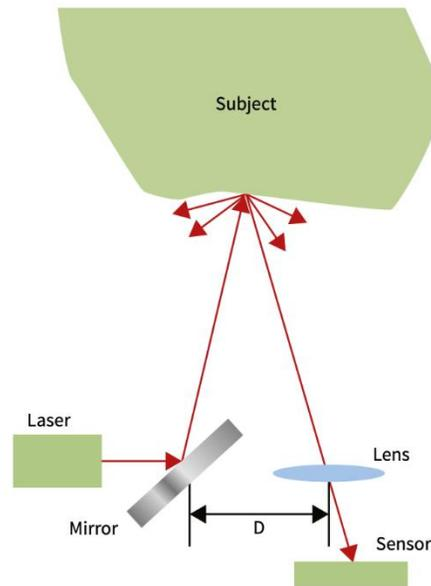
Figure 1-11: Working principle of triangulation scanners (Historic England, 2018)
