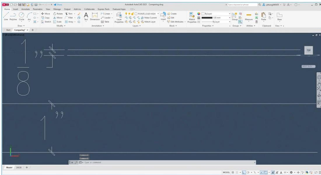
Figure 5-24: Measuring point thickness with dimensional tool. RTC 360 point cloud thickness is 1/8",
