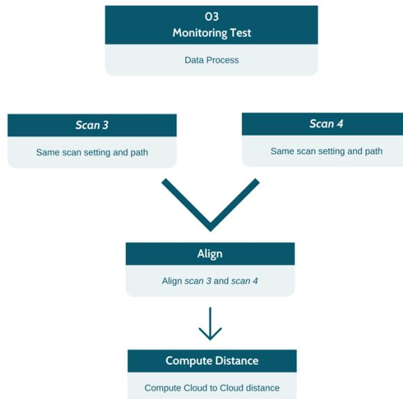
Figure 4-73: Monitoring data process work flow
