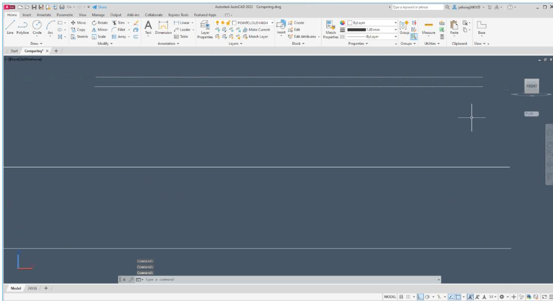
Figure 5-23: Tracing top and bottom points in section 2 with line command
