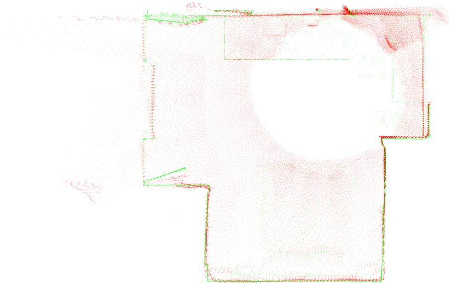
Figure 5-12: Manual align smartphone scans (red) with professional scans (green).
