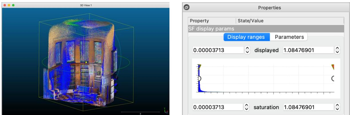
Figure 4-83, Cloud-to-cloud distance visualization from CloudCompare for *scan 3* and *scan 4*.
