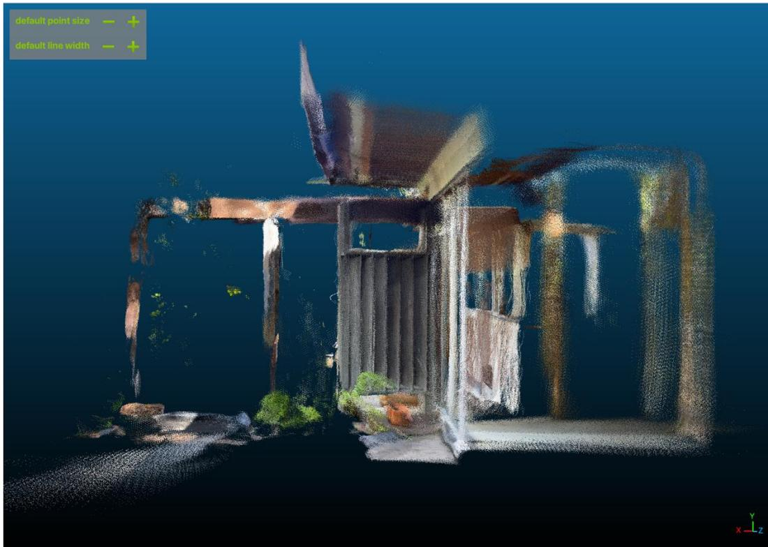
Figure 6-8: iPhone scanned front yard at Reunion House with a “spider leg” feature.
