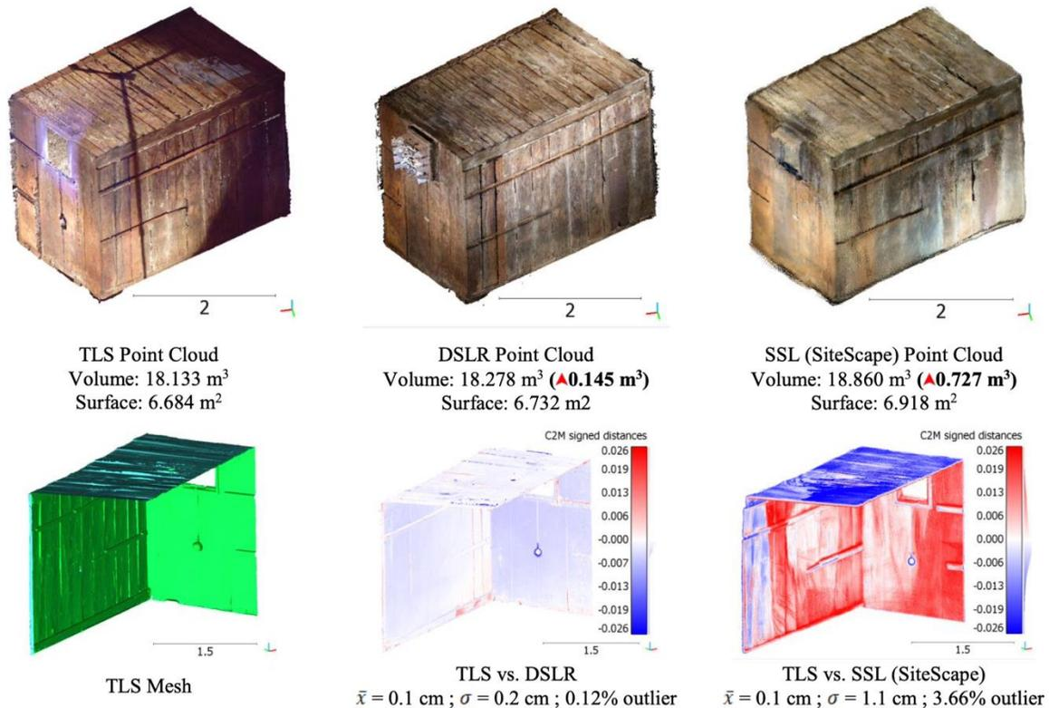
Figure 2-12: Data comparison with TLS, DSLR, and SSL (smartphone) (Spreafico et al., 2021).
