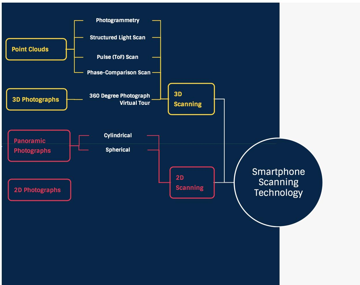
Figure 1-18: Smartphone Scanning Methods
