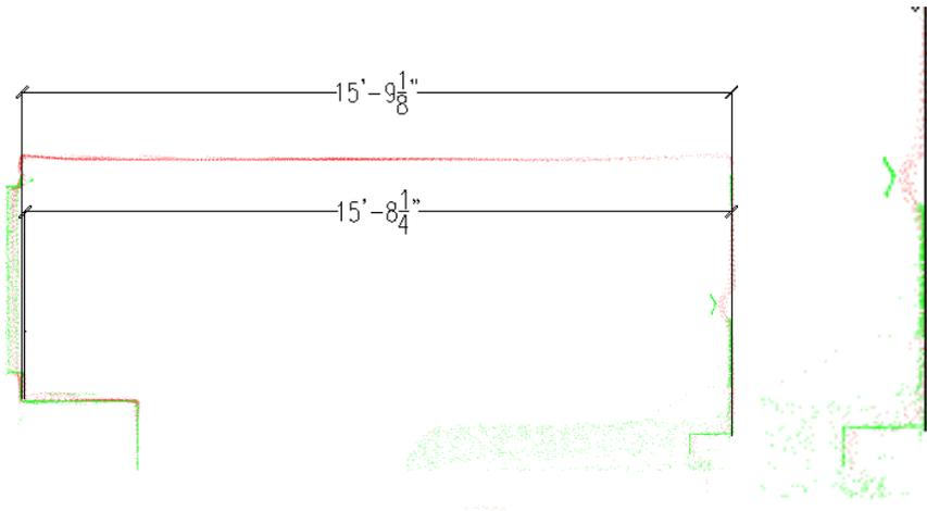
Figures 6-5: Low density iPhone scan (red) and RTC 360 scan (green) section 1 (left), and detail (right).
