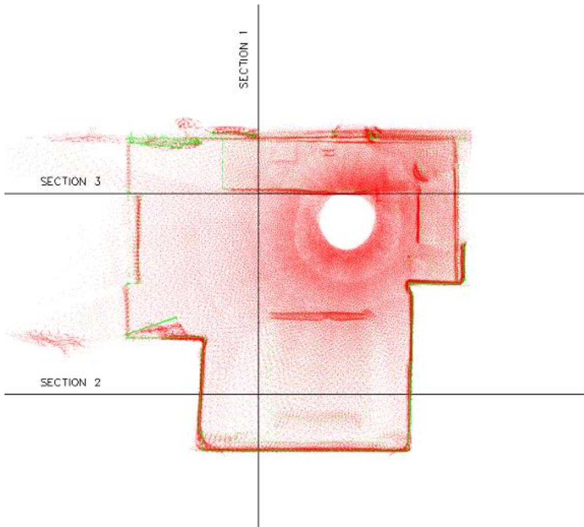
Figure 7-5: Overlapping professional scanner point cloud with iPhone scanned point cloud.
