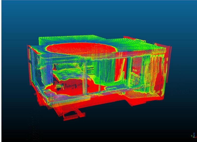
Figure 7-7: Cloud to cloud distance computation result in CloudCompare
