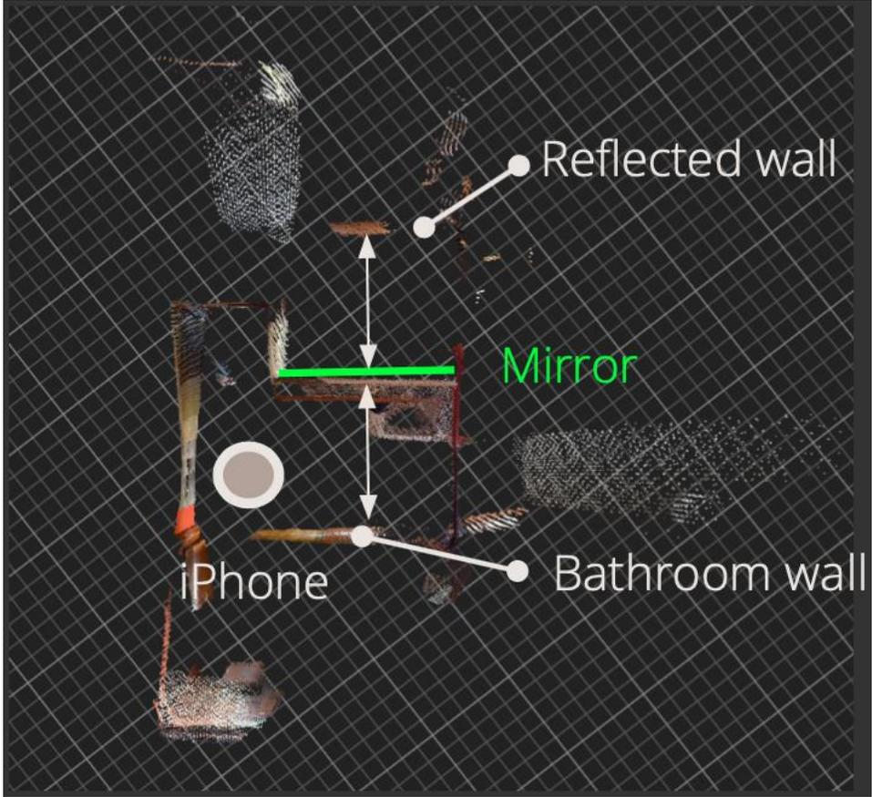
Figure 6-6: Mirror reflection captured by smartphone
