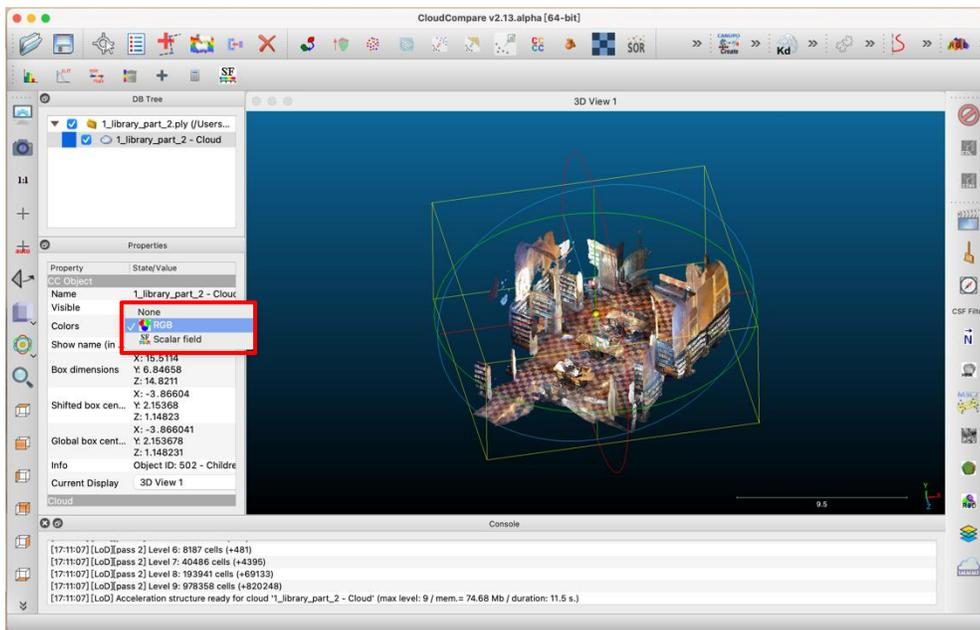
Figures 4-55 and 4-56: After merge view in scalar field and how to change to RGB color
