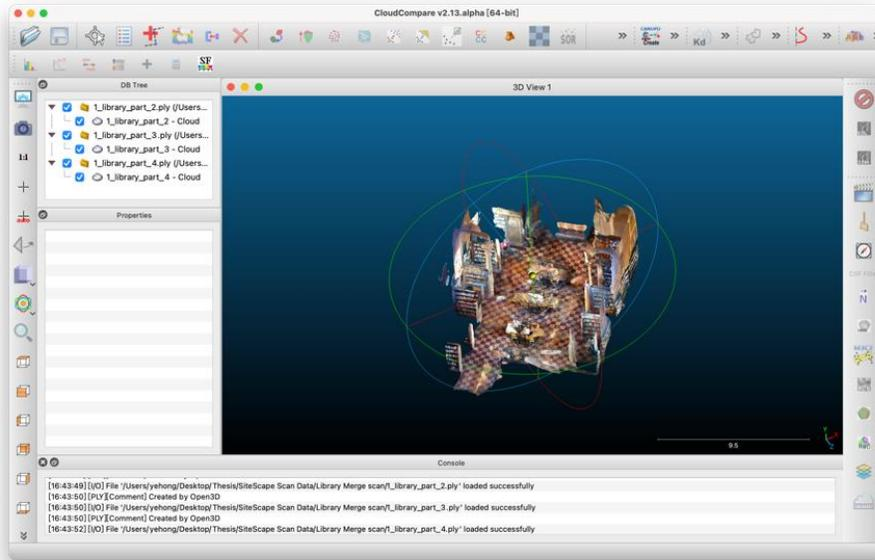
Figures 4-50, 4-51, and 4-52: Point clouds automatically registered and merged
