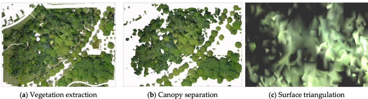
Figure 2-2: The three major processing steps of PCs. (a) The vegetation was extracted by using SVIs. (b) Grass was separated from the canopy using CSF. (c) The separated canopy PCs were triangulated using Delaunay triangulation. (Zhang et al., 2022)
