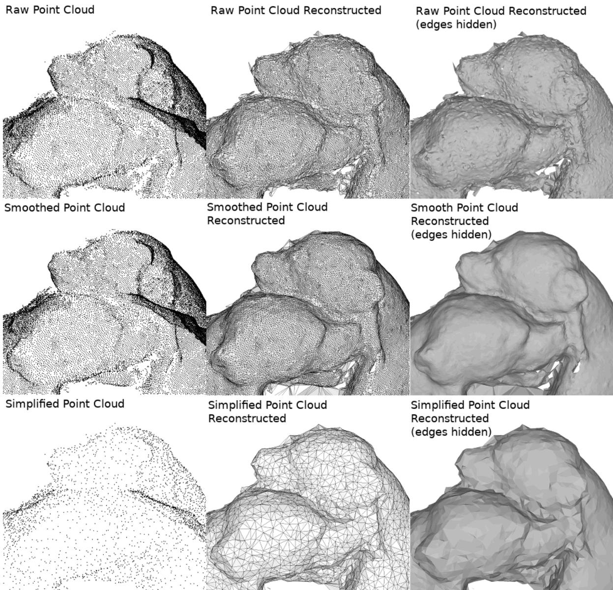
Figure 1-10: Same point cloud data with different processing in reconstructing surface (Giraudot, 2022)
