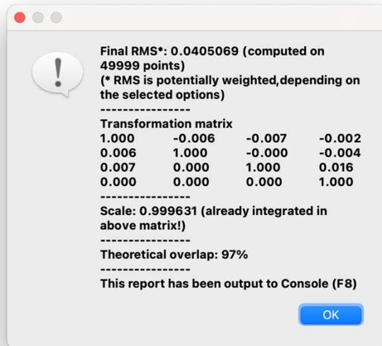
Figure 4-79: Result of aligning *scan 3* and *scan 4*
