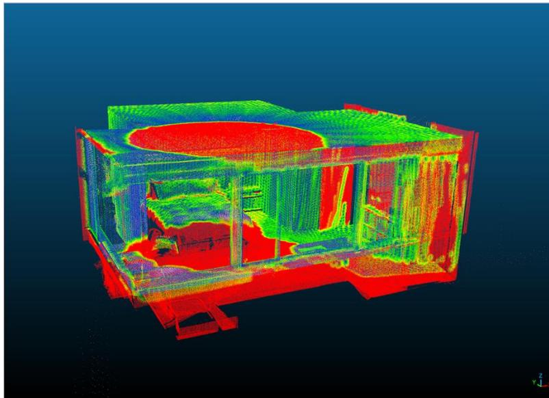
Figure 6-13: Cloud to cloud distance computation result in CloudCompare
