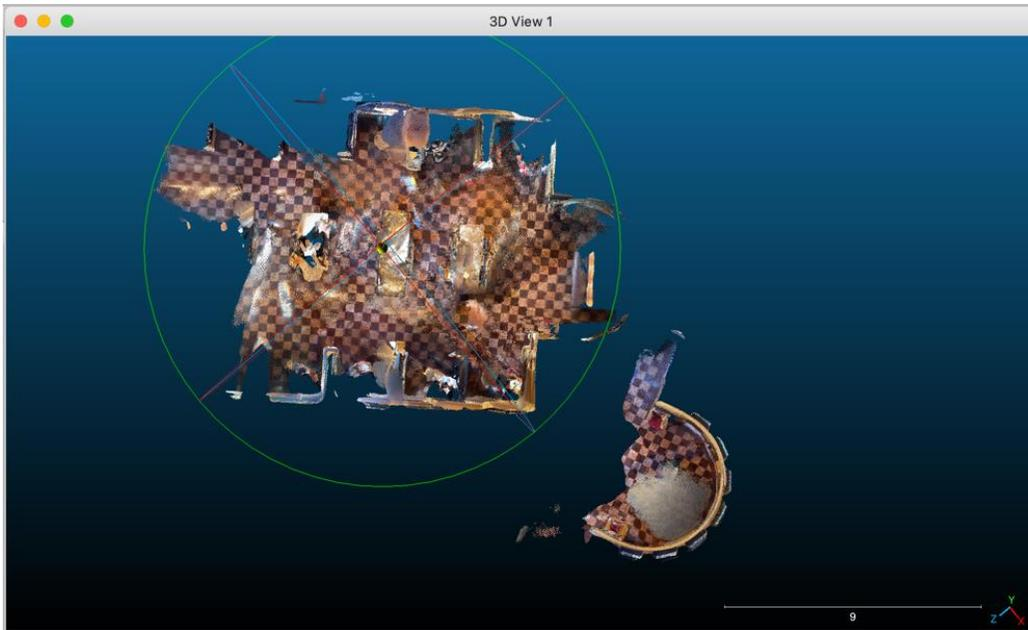
Figure 4-63: Move to-be-aligned point cloud away from reference point cloud
