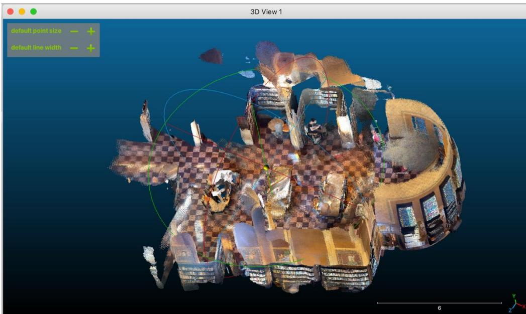
Figures 4-67 and 4-68: Pick equivalent points on both to-be-aligned and reference entities, and align result
