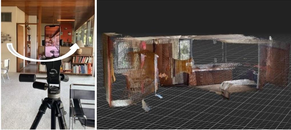
Figure 5-5 and 5-6: Smartphone scan moving path and scan result
