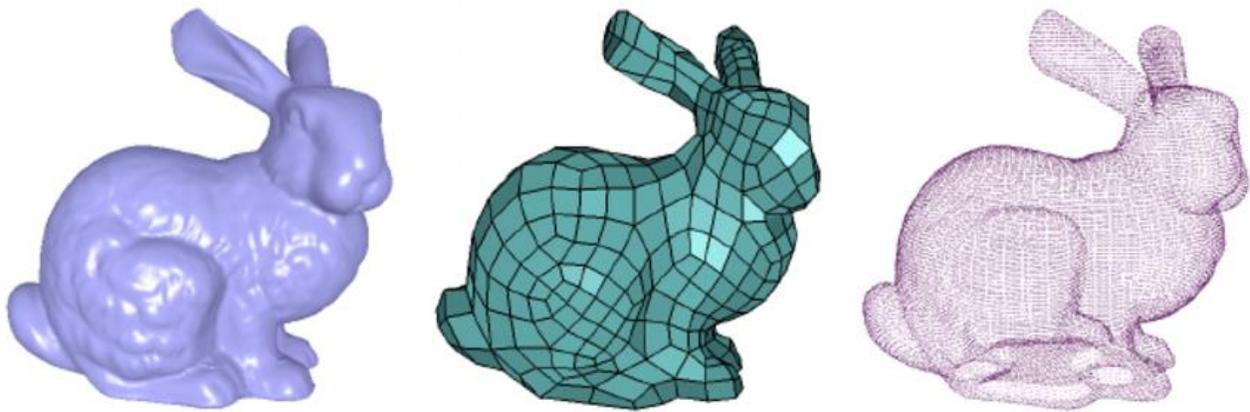
Figure 1-8: Point Clouds, Control Mesh, Result visualization of a rabbit (Yoon, 2006)
