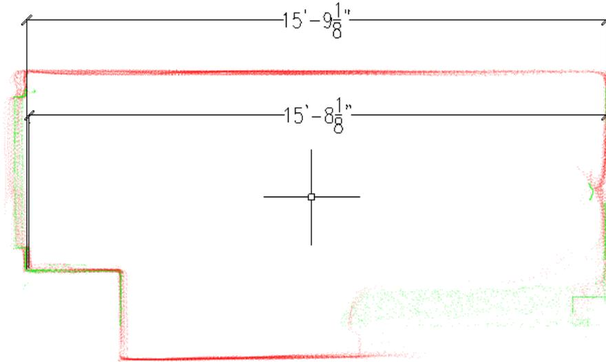
Figure 5-17: Measurement example (room width) of iPhone acquired low point density merge scan (red) and professional scan (green) in section 1
