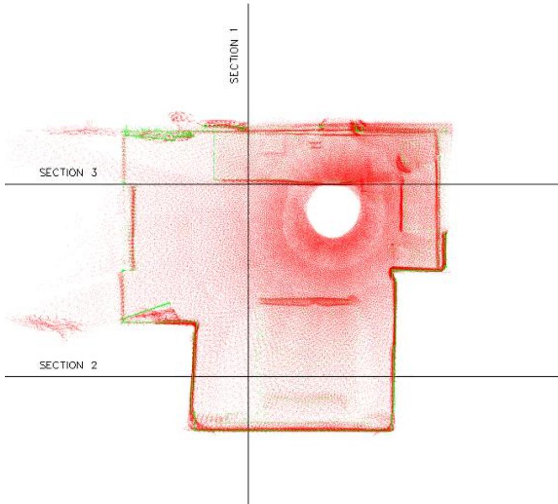
Figure 6-2: Smartphone scans were manually aligned with professional scanners' scan in AutoCAD.
