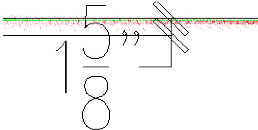
Figure 5-26: Ceiling detail in low point density scan section 2. Green representing RTC 360 scanner data, red representing iPhone scanned data. The thickness of scanner points is 1/8"; the thickness of iPhone scanned points is 1 5/8"
