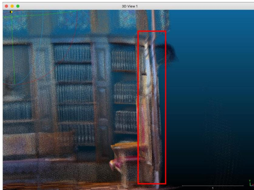
Figure 4-26: Double layer of points in *scan 2*
