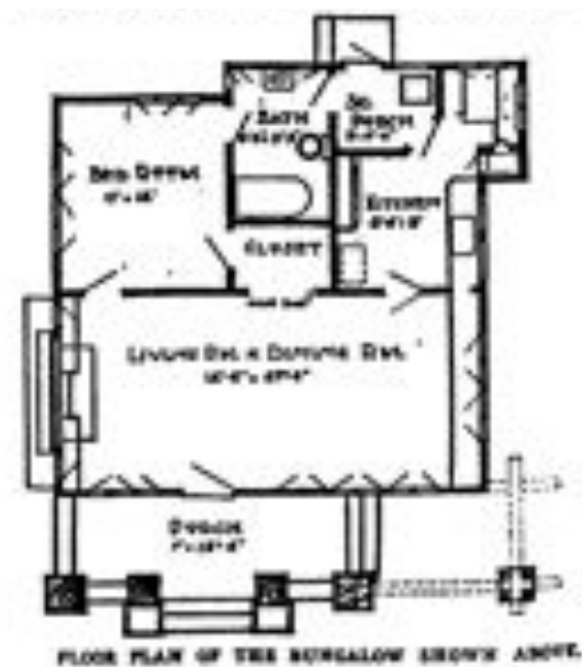
Figure 1.6: California Bungalow Floor Plan. Courtesy of Byers, "The Bungalow Court Idea Shown in Practical Operation."
