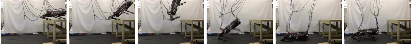
Fig. 7: Motion snapshots from a successful jump down from a desk with the height of 30 inches.
