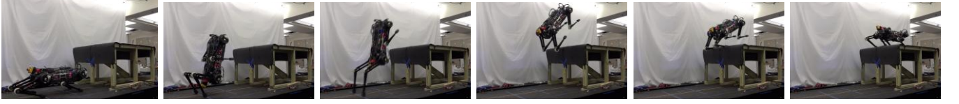
Fig. 6: Motion snapshots from a successful jump on a desk with the height of 30 inches.
