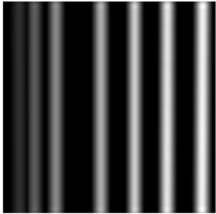
Fig.13. The finest line is very fuzzy on the result as bigger Gauss core parameter \sigma is chosen.
