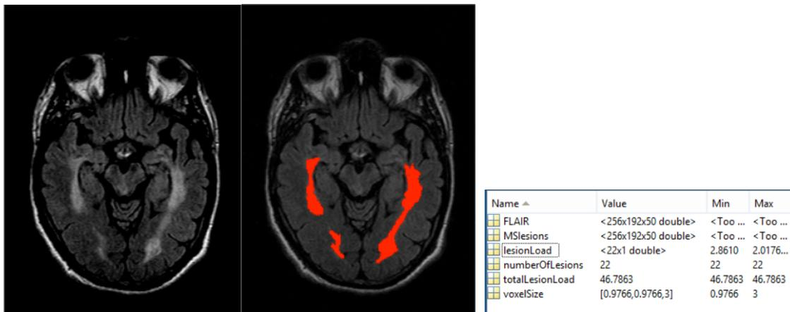
Figure 3. Raw MATLAB output of MS CAD. Left: original FLAIR axial image. Middle: lesion contour overlaid on the FLAIR image. Right: MATLAB outputs. lesionLoad includes individual lesion volumes, numberOfLesions indicates that there are 22 unique lesion bodies in this study, and totalLesionLoad is the sum of all lesion volumes.
