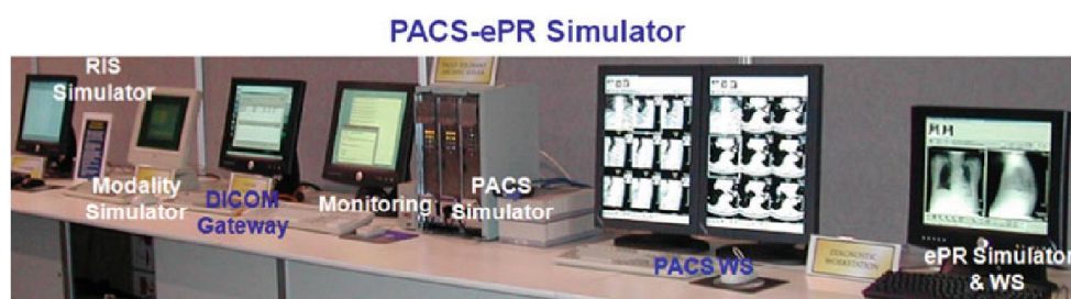
Fig. 2 The PACS–ePR simulator shown at an RSNA exhibits. Left to right RIS simulator, modality simulator, DICOM gateway, monitoring system of the data flow of the PACS–ePR simulator operation, PACS simulator, PACS WS, and Web-based ePR simulator and WS [2,3]
