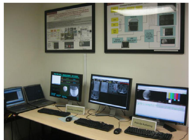
Fig. 14 The IAS ePR simulator in the laboratory environment simulating the pre-op and intra-op of a MISS surgery. Right to left two pre-op displays, an intra-op live display and two DVD devices feeding simulating data to the intra-op display
