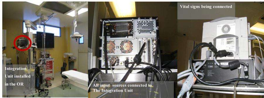
**Figure 12.** Integration Unit (IU, left inside the red ring) installed in the OR connected to different input sources. (Middle: Input units cables are connected to the back of the IU; Right: Vital Signs device is being connected.).
