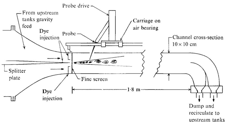
FIGURE 1. Schematic diagram of apparatus. (Not to scale.)
