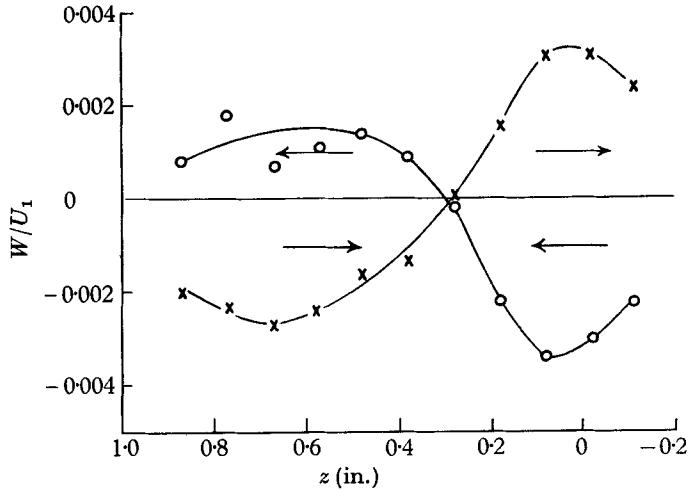
FIGURE 35. Spanwise distribution of spanwise component of mean velocity for 'natural' transition:  $U_1/\nu = 4.6 \times 10^5$  ft.<sup>-1</sup>. 5.75 ft. from leading edge:  $\circ$ ,  $0.3\delta$ ;  $\times$ ,  $0.1\delta$ .
