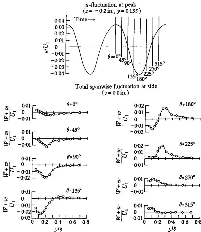
FIGURE 15. Distributions of the total spanwise component of velocity across boundary layer. Station B: 145 c/s wave,  $U_1/\nu = 3.1 \times 10^6$  ft.<sup>-1</sup>.
