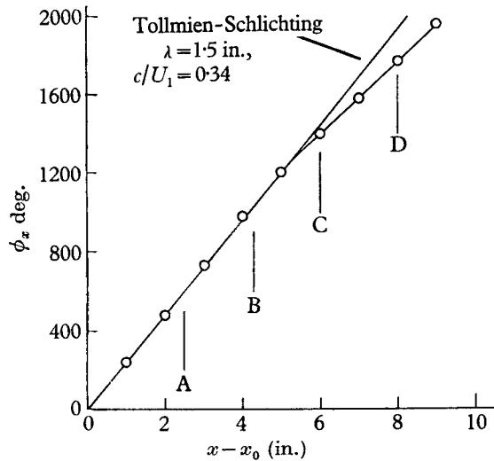
FIGURE 7. Phase of  $u$ -fluctuation in downstream direction: 145 c/s wave,  $y = 0.045$  in.,  $U_1/\nu = 3.1 \times 10^5$  ft.<sup>-1</sup>.
