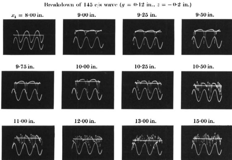
FIGURE 21. Oscillograms of  $u$ -fluctuation illustrating breakdown process; time increasing from left to right, decreasing velocity in downward direction;  $U_1/\nu = 3.1 \times 10^5$  ft.<sup>-1</sup>.
