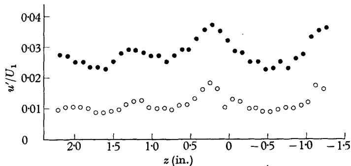
FIGURE 33. Spanwise distributions of intensity of  $u$ -fluctuation for 'natural' transition:  $y = 0.052$  in.,  $U_1/\nu = 4.6 \times 10^5$  ft.<sup>-1</sup>. ○, 5.5 ft. from leading edge; ●, 5.75 ft. from leading edge.
