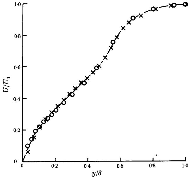
FIGURE 23. Mean velocity distributions across boundary layer at position of initial breakdown for two different wave frequencies and Reynolds numbers per foot. O, 145 c/s,  $U_1/\nu = 3.1 \times 10^5$  ft.<sup>-1</sup>; x, 65 c/s,  $U_1/\nu = 1.9 \times 10^5$  ft.<sup>-1</sup>.
