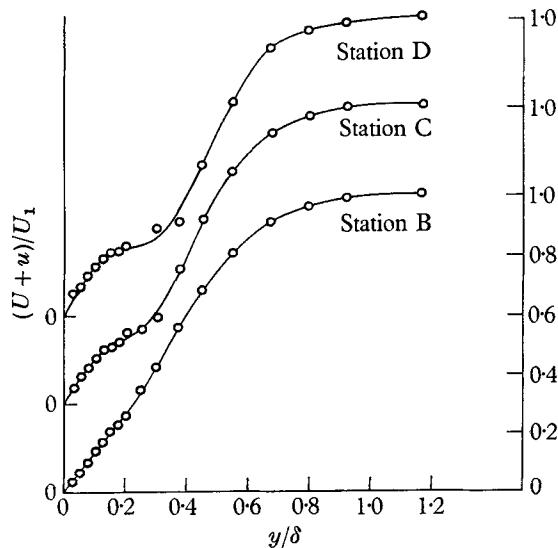
FIGURE 30. Instantaneous velocity distributions across boundary layer:
