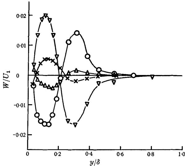
FIGURE 12. Distributions of spanwise component of mean velocity across boundary layer. 145 c/s wave,  $U_1/\nu = 3.1 \times 10^5$  ft.<sup>-1</sup>. Station B:  $\Delta$ ,  $z = 0.0$  in.;  $\times$ ,  $z = 0.4$  in. Station C:  $\circ$ ,  $z = 0.0$  in.;  $\nabla$ ,  $z = -0.4$  in.
