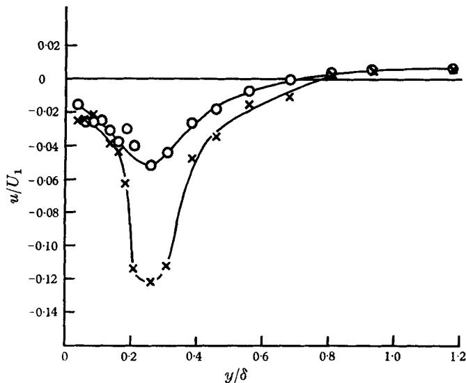
FIGURE 17. Distribution of  $u$ -fluctuation across boundary layer at time  $\theta = 180^\circ$ : 145 c/s wave,  $U_1/\nu = 3.1 \times 10^5 \text{ ft.}^{-1}$ .  $\circ$ , Station B:  $z = 0.0 \text{ in.}$ ,  $\theta = 180^\circ$ .  $\times$ , Station C:  $z = 0.0 \text{ in.}$ ,  $\theta = 180^\circ$ .
