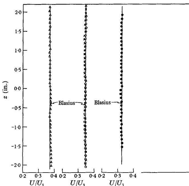
FIGURE 1. Spanwise distribution of mean velocity at different distances downstream from vibrating ribbon:  $y = 0.042$  in.,  $U_1/\nu = 3.1 \times 10^5$  ft.<sup>-1</sup>. Ribbon and spacers:  $\Delta$ ,  $x_1 = 1$  in.;  $\circ$ ,  $x_1 = 7$  in.;  $\bullet$ ,  $x_1 = 10$  in. No ribbon and spacers:  $\times$ ,  $x_1 = 7$  in.
