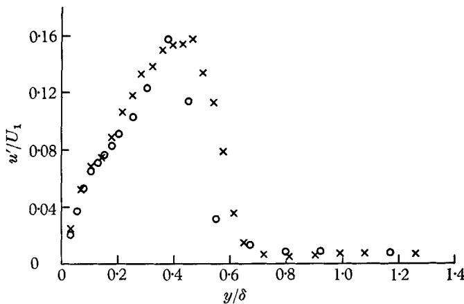
FIGURE 24. Distribution of intensity of  $u$ -fluctuation across boundary layer at position of initial breakdown for two different wave frequencies and Reynolds numbers per foot. O, 145 c/s,  $U_1/\nu = 3.1 \times 10^5$  ft. $^{-1}$ ; x, 65 c/s,  $U_1/\nu = 1.9 \times 10^5$  ft. $^{-1}$ .
