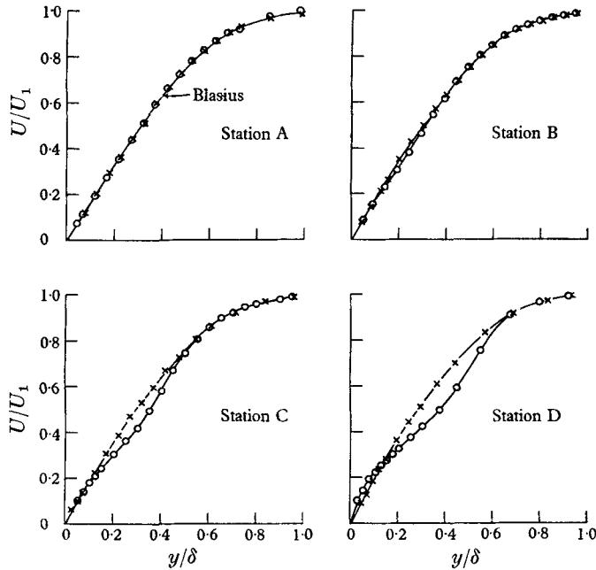
FIGURE 10. Mean velocity distributions across boundary layer at peak and valley: 145 c/s wave,  $U_1/\nu = 3.1 \times 10^5$  ft.<sup>-1</sup>.  $\circ$ ,  $z = -0.2$  in.;  $\times$ ,  $z = -0.75$  in.
