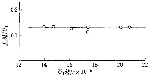
FIGURE 29. Non-dimensional plot of 'hairpin' eddy frequency.
