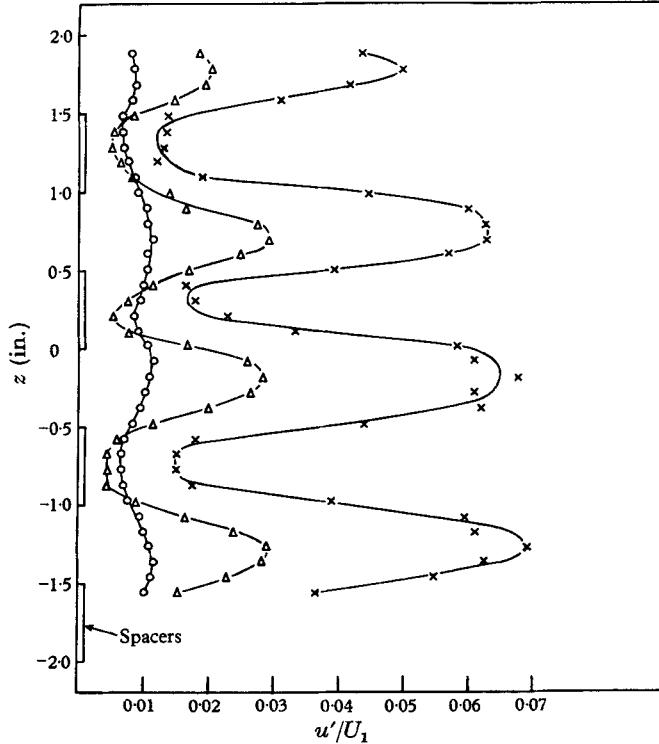
FIGURE 2. Spanwise distributions of intensity of  $u$ -fluctuation at different distances downstream from vibrating ribbon: 145 c/s wave,  $y = 0.042$  in.,  $U_1/\nu = 3.1 \times 10^5$  ft.<sup>-1</sup>.  $\circ$ ,  $x_1 = 3$  in.;  $\triangle$ ,  $x_1 = 6$  in.;  $\times$ ,  $x_1 = 7.5$  in.
