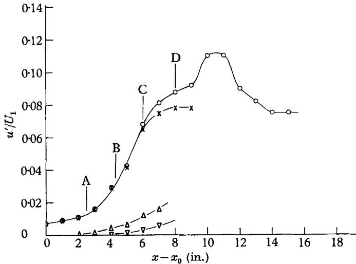
FIGURE 9. Harmonic content of  $u$ -fluctuation: 145 c/s wave,  $y = 0.045$  in.,
