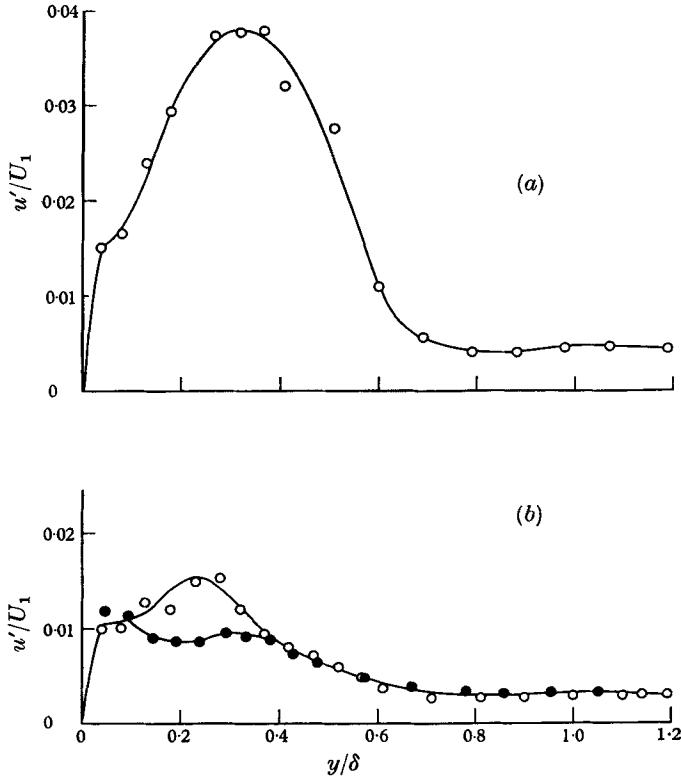
FIGURE 34. Distribution of intensity of  $u$ -fluctuation across boundary layer for 'natural' transition:  $U_1/\nu = 4.6 \times 10^5$  ft.<sup>-1</sup>. (a) 5.75 ft. from leading edge:  $\circ$ ,  $z = 0.25$  in.; (b) 5.5 ft. from leading edge:  $\circ$ ,  $z = 0.25$  in.;  $\bullet$ ,  $z = -0.5$  in.
