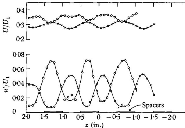
FIGURE 13. Spanwise distribution of mean velocity and intensity of  $u$ -fluctuation at two different Reynolds numbers per foot: 65 c/s wave,  $x = 3.75$  ft.  $\circ$ ,  $U_1/\nu = 3.1 \times 10^5$ ,  $y = 0.043$  in.;  $\times$ ,  $U_1/\nu = 1.9 \times 10^5$ ,  $y = 0.048$  in.
