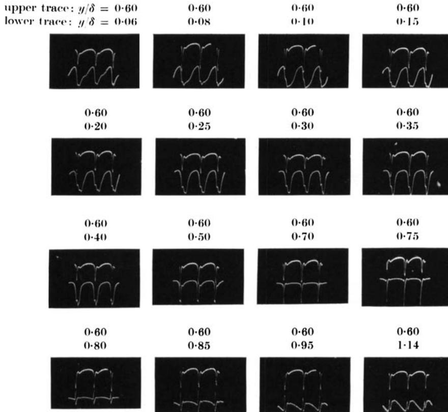
FIGURE 26. Oscillograms of simultaneous  $u$ -fluctuations illustrating phase and extent of breakdown in  $y$ -direction: primary wave 145 c/s; time increasing from left to right, decreasing velocity in downward direction;  $U_1/\nu = 3.1 \times 10^5 \text{ ft.}^{-2}$ .
