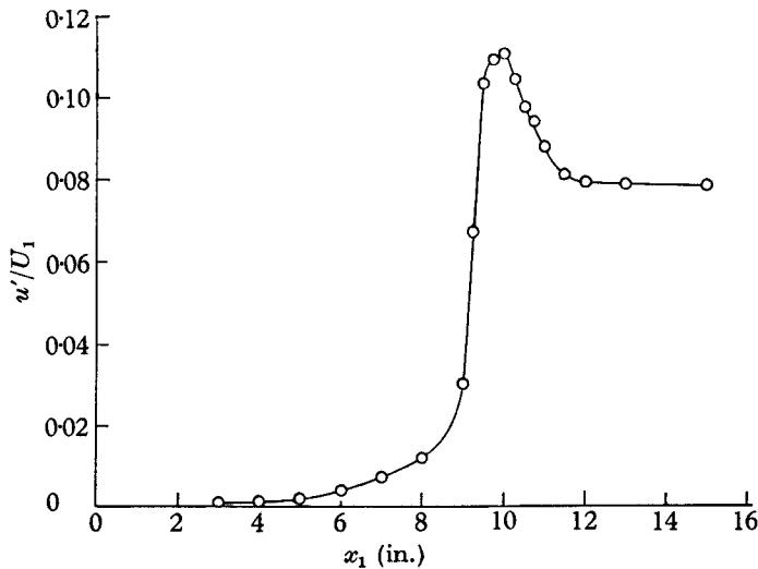
FIGURE 22. Growth in intensity of  $u$ -fluctuation associated with the oscillograms of figure 21: 145 c/s wave,  $y = 0.12$  in.,  $z = -0.2$  in.,  $U_1/\nu = 3.1 \times 10^5$  ft.<sup>-1</sup>.
