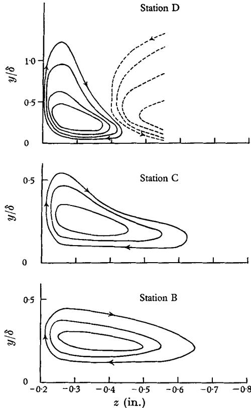
FIGURE 19. Schematic representation of streamlines in  $(y, z)$ -plane:
