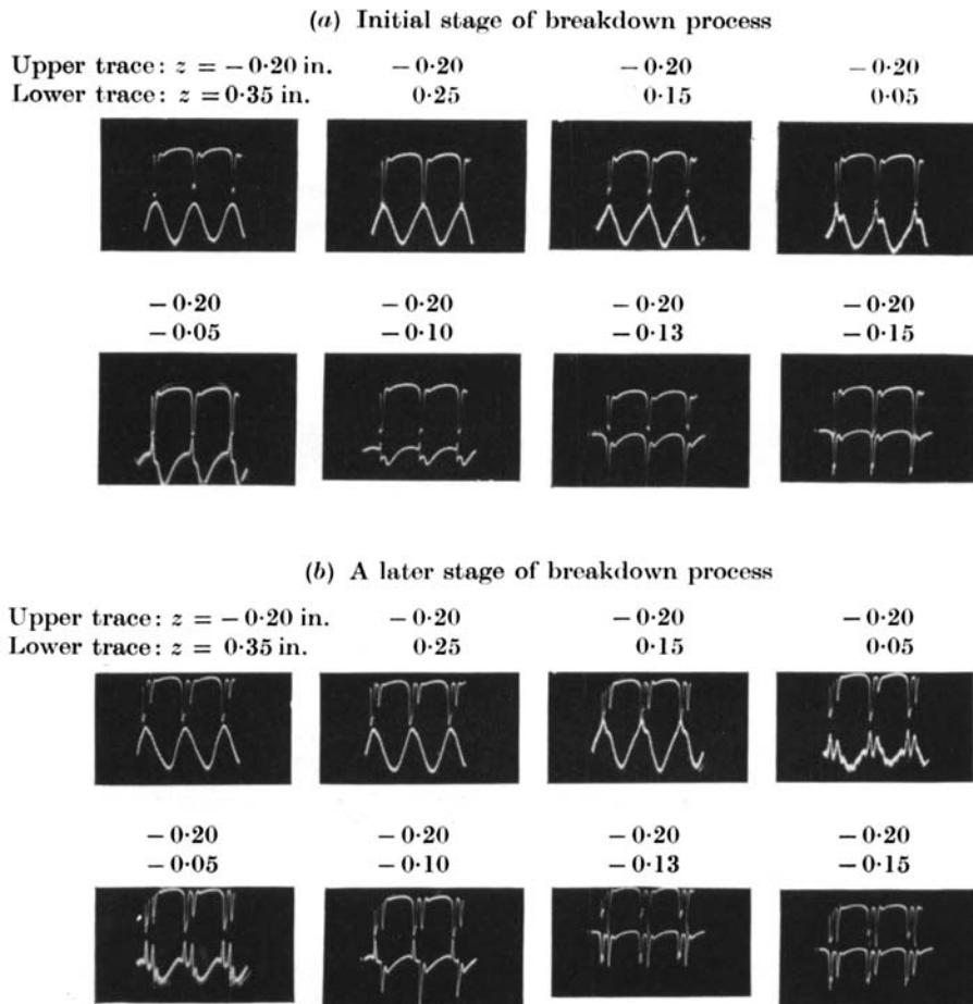
FIGURE 25. Oscillograms of simultaneous  $u$ -fluctuations illustrating phase and extent of breakdown in  $z$ -direction: primary wave 145 c/s; time increasing from left to right, decreasing velocity in downward direction;  $U_1/\nu = 3.1 \times 10^5$  ft.<sup>-1</sup>.
