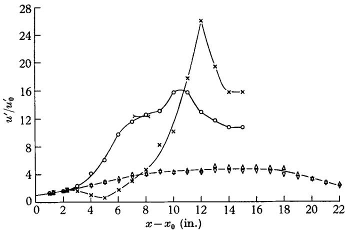
FIGURE 3. Wave growth at peak and valley: 145 c/s wave,  $y = 0.045$  in.,  $U_1/\nu = 3.1 \times 10^5$  ft.<sup>-1</sup>. Peak:  $\triangle$ ,  $u'_0/U_1 = 0.0008$ ;  $\circ$ ,  $u'_0/U_1 = 0.007$ . Valley:  $\nabla$ ,  $u'_0/U_1 = 0.0007$ ;  $\times$ ,  $u'_0/U_1 = 0.005$ .  $>—<$ , Breakdown.
