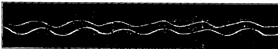
A. Comparison of wall cell (fainter record) and wall plate. Air speed, 40 ft./sec. Time breaks, 0.034 sec. apart. Wind tunnel motor, 300 revolutions per minute. Frequency of blade impulses, 20 per second. Length of air column on wall plate, 19.3 inches; natural frequency, 26.8 per second
