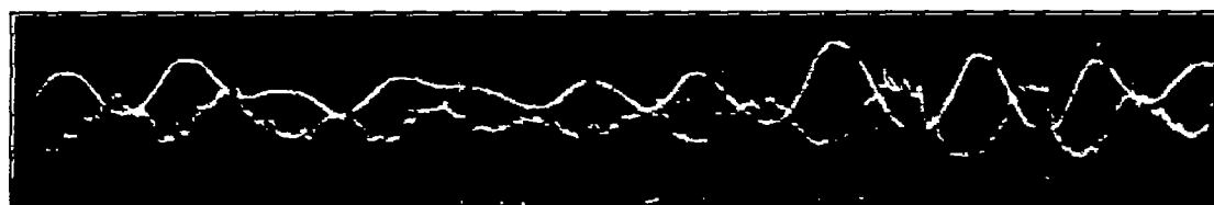
C. Comparison of wall cell (fainter record) and wall plate. Air speed, 60 ft./sec. Time breaks, 0.03 sec. apart. Wind tunnel motor, 450 revolutions per minute. Frequency of blade impulses, 30 per second. Length of air column on wall plate, 19.3 inches; natural frequency, 26.8 per second.
