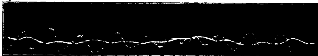
C. Comparison of static of large Pitot tube and wall cell; 43.3 inches of \frac{1}{4} -inch tubing; 66 ft./sec. Time breaks, 0.03 sec. apart. Wind tunnel motor, 495 revolutions per minute. Frequency of blade impulses, 33 per second
