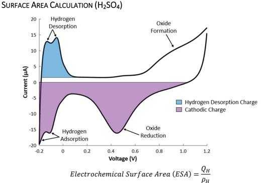
Hydrogen Desorption Charge  $(Q_H) = time integral of hydrogen desorption current$ Characteristic charge density of monolayer of $hydrogen atoms adsorbed to polycrystalline Pt <math>(\rho_H) = 210 \frac{\mu C}{cm^2}$
