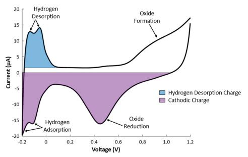
$\begin{array}{l} \textit{Charge Storage Capacity}\left(\textit{CSC}\right) = \frac{Q_{\textit{cathodic}}}{GSA}\\ \textit{Cathodic Charge}\left(Q_{\textit{cathodic}}\right) = time \ \textit{integral of cathodic current}\\ \textit{Geometric Surface Area}\left(GSA\right) = \textit{geometric area of electrode} \end{array}$
