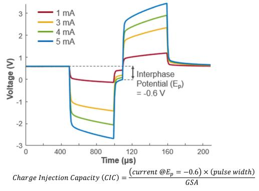
Geometric Surface Area (GSA) = geometric area of electrode
