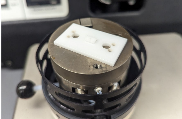
Figure 6: The chip holder should sit on the wire bonder workstage, with the hole lined up with the workstage's vacuum.
