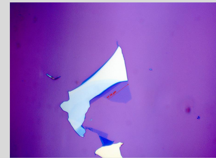
Measuring length of graphene samples early in the extraction process.
