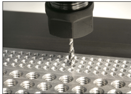
The Haas-built BT30 taper inline direct-drive spindle provides 15,000 rpm for high-speed milling, and allows rigid tapping at speeds up to 5000 rpm.
